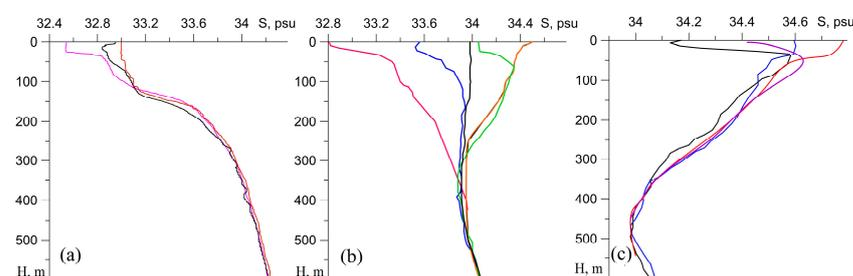
**Figure 2.** Typical vertical distribution of salinity in areas with different signs of freshwater balance: (a) positive; (b) transition zone; (c) negative. Salinity profiles are located between 160° E and 160° W: (a) 48° N; (b) 43° N; (c) 38° N.
