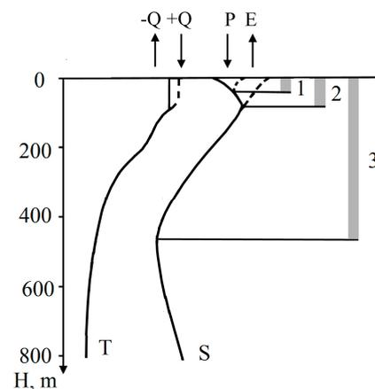
**Figure 1.** Characteristic vertical distribution of temperature and salinity in the arid zone of the ocean. Explanation: 1—active layer of synoptic time scale; 2—active layer of seasonal time scale; 3—active layer of great (geological) time scale.
